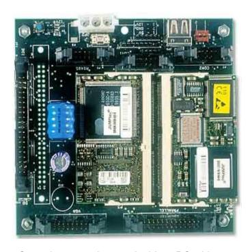
Sometimes you just can't ship a PC with every order. We designed a custom computer to control the environment in the cargo bay of the Space Shuttle.
